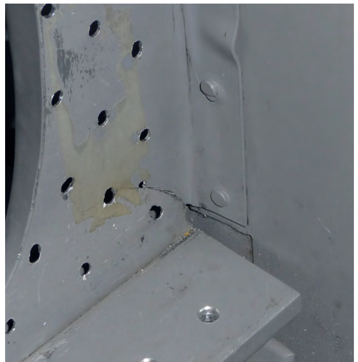
This picture of the wing forward attachment was taken from the foot pedals so you're looking at the inside of the bracket. This riveting is definitely below par and needs to be replaced. (Photo: Roy Holder)
